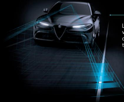
Lane Keep Assist alerts the driver if the vehicle is straying out of its lane and provides a corrective action to help automatically correct the vehicle's path and direct it back into the lane.
